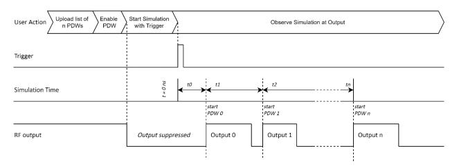
Figure 2: List mode timing concept with relative Time Mode. PDWs are applied at their dedicated start times. Figure not to scale.
