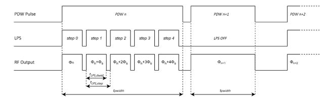
Figure 9: Graphical representation of pulse behavior with Linear Phase Sweep. Graph features PDW Pulse defined by START\_TIME and PULSE\_WIDTH, LPS pulse defined by SWEEP\_DWELL and SWEEP\_STEP and the resulting pulse and phase behavior at the RF output of the device. Figure not to scale.
