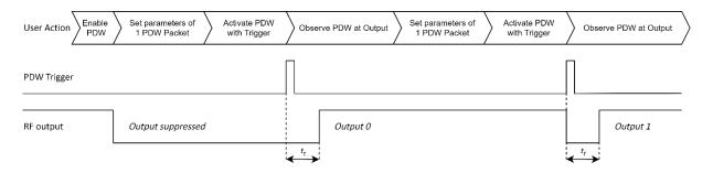
Figure 4: Single mode concept with trigger. Figure not to scale.
